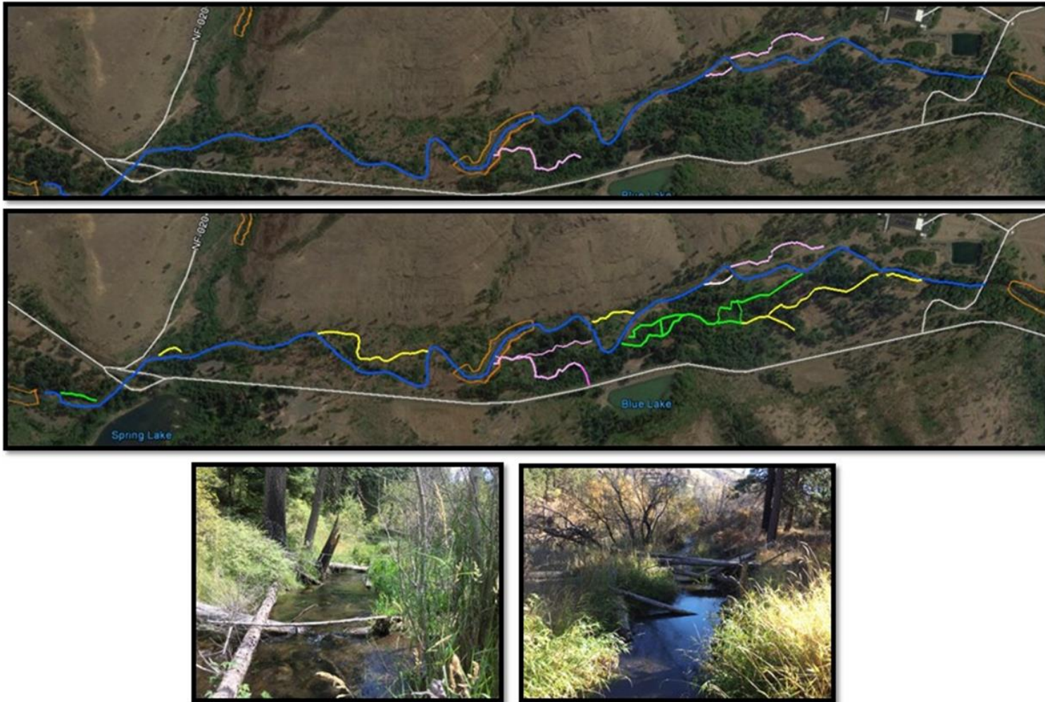
Figure 6: The program partners within the Tucannon have used side channel re-connection actions to reconnect floodplain and increase River Complexity. The upper map illustrates side channel reconnection in one project reach in the Tucannon (upper pre-project and lower post project, with the green lines being perennial, yellow being ephemeral and pink being reconnected tributaries). The lower pictures illustrate channel conditions within reconnected side channel reaches.
